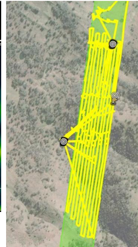
Thermal drone survey flight lines
