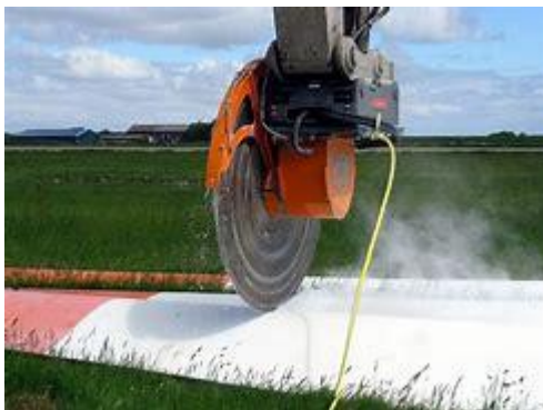
Cutting up end-of-life wind turbine blades
