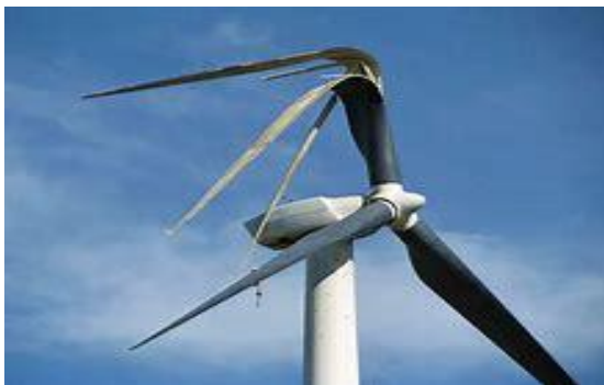
Lightning strike shuts down wind turbine
